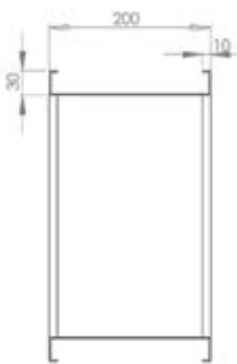
Flange joint for TDC (T) connection (optional) for ductwork installation
